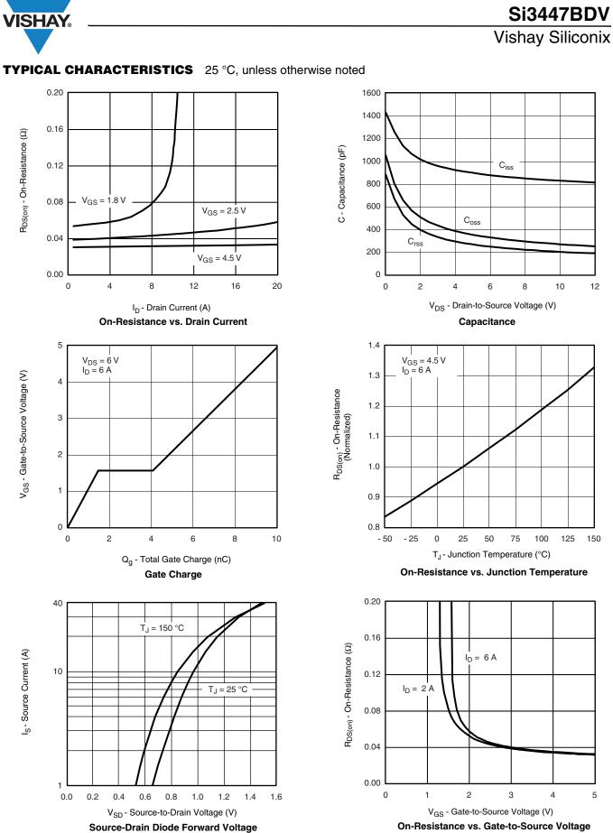
Source-Drain Diode Forward Vo
