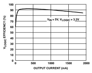
FIGURE 4. VLOGIC EFFICIENCY vs OUTPUT CURRENT
