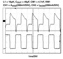
FIGURE 3.  $A_{\mbox{\scriptsize VDD}}$  TRANSIENT RESPONSE
