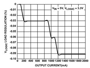
FIGURE 8. V<sub>LOGIC</sub> LOAD REGULATION vs OUTPUT CURRENT
