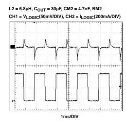
FIGURE 6. VLOGIC TRANSIENT RESPONSE
