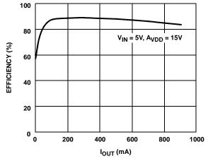
FIGURE 1.  $A_{VDD}$  EFFICIENCY vs  $I_{OUT}$
