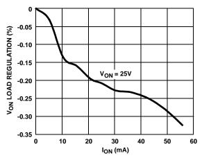
FIGURE 7. VON LOAD REGULATION vs ION
