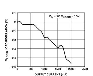
FIGURE 5. VLOGIC LOAD REGULATION vs OUTPUT CURRENT
