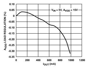
FIGURE 2.  $A_{VDD}$  LOAD REGULATION vs  $I_{OUT}$
